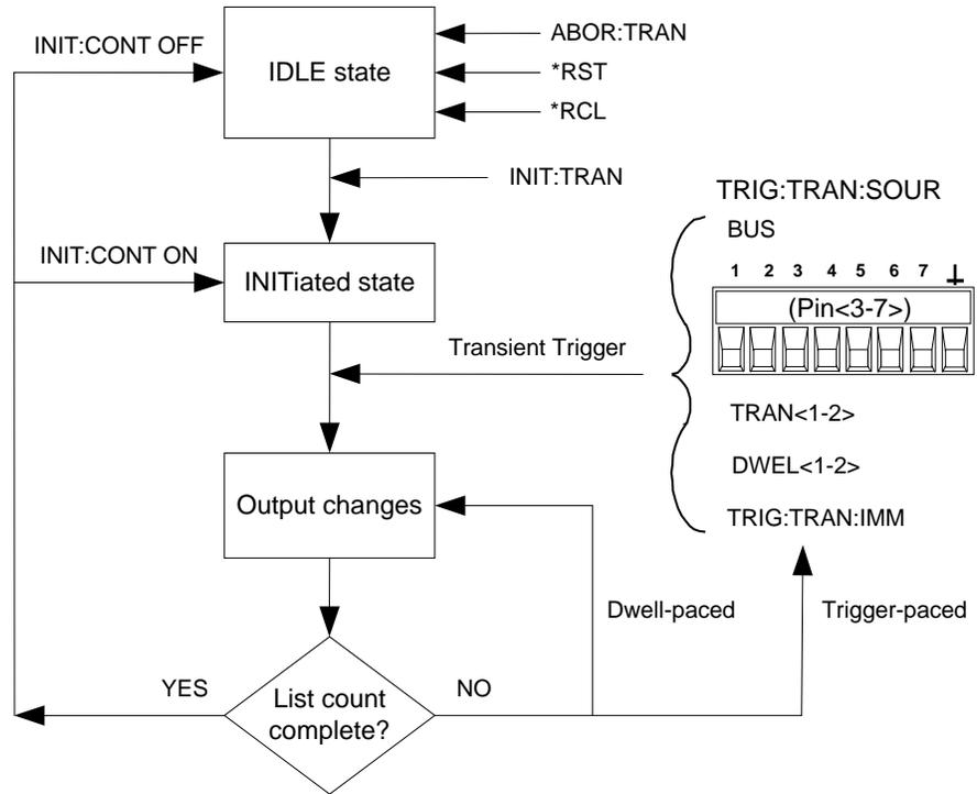
If you need the curve lists to closely follow external events, the lists can be paced by external trigger signals. With trigger-pacing, the lists advance one curve for each trigger received. Select a trigger source from the available trigger sources. With a trigger-paced list, you do not need to program a dwell time for each curve.
