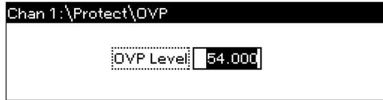
Press the **Channel** key at any time to select a different output channel. This can save time because you can directly access the OVP control of each channel without having to navigate through the menu levels.
