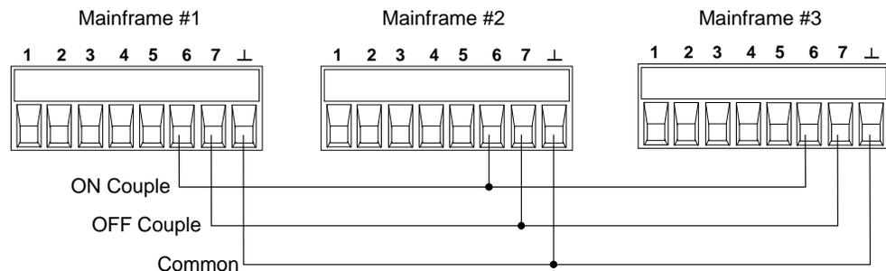
Output coupling must be enabled on all mainframes that will have one or more of their outputs coupled.
