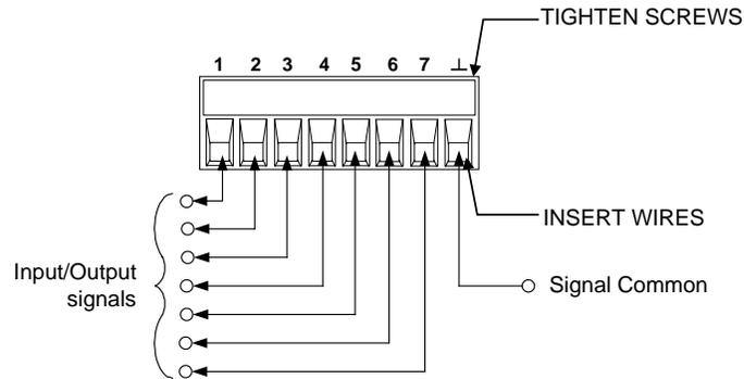
The digital control connector accepts wires sizes from AWG 14 to AWG 30. Note that wire sizes smaller than AWG 24 are not recommended. Disconnect the connector plug to make your wire connections.
