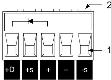
The output connector was shipped with two local sense jumpers. With these sense jumpers installed (from +s to +; from -s to -), the unit senses and regulates its output voltage directly at the output terminals. This causes the voltage at the load to be somewhat lower due to the voltage drop in the load leads. In applications where voltage regulation at the load is critical, remote sensing may be required as explained later in this chapter.
