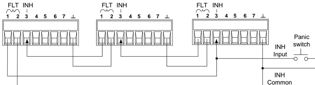
As shown in the previous figure, when the Fault outputs and Inhibit inputs of several mainframes are daisy-chained, an internal fault condition in one of the mainframes will disable all of them without intervention by either the controller or external circuitry. You must select the **same** polarity (either positive or negative) for all FLT and INH pins in the daisy chain.
