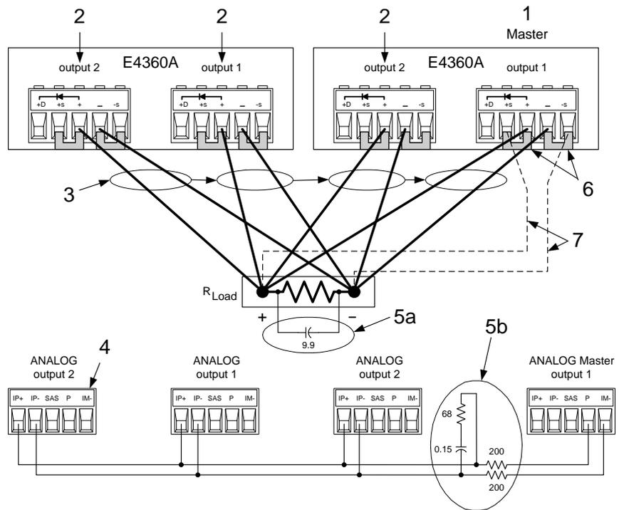
As shown in the following table, the capacitor values required for the two compensation methods depend on the number of follower outputs that are paralleled.
