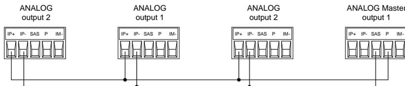
As in Fixed mode, you must specify which output channel is the master and which outputs are followers. Refer to chapter 4 under “Configuring Paralleled Outputs”. In SAS mode, the same model parameters or list step must be in effect for each output channel. If lists are used, each output must get the same list steps and triggering to cause the outputs to change steps at the same time. In Table mode, the same user-table must be activated for all outputs.
