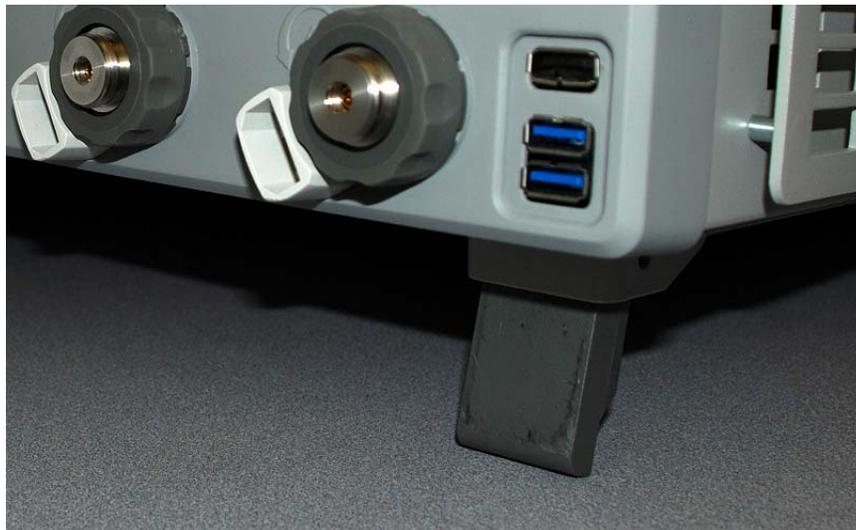
**Figure 4** Flip-Out tabs under front feet
