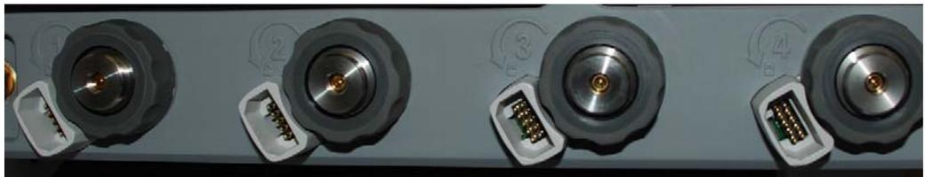
**Figure 3** V-Series oscilloscope probe connectors
