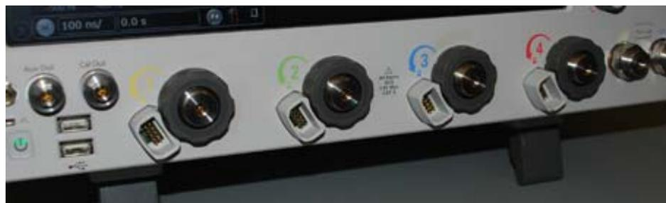
**Figure 3** Z-Series oscilloscope probe connectors
