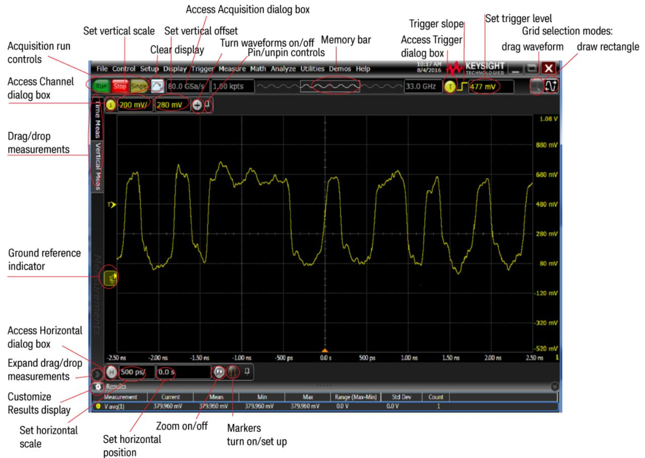
Figure 11 Infiniium oscilloscope display
