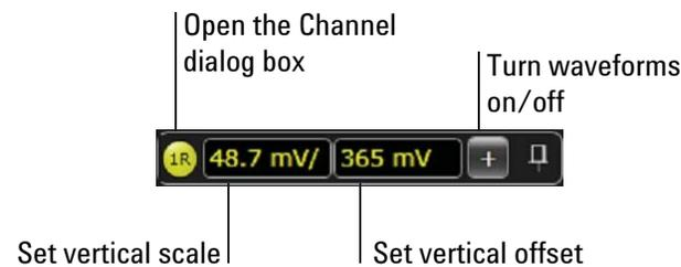
**Figure 19** User interface vertical controls
