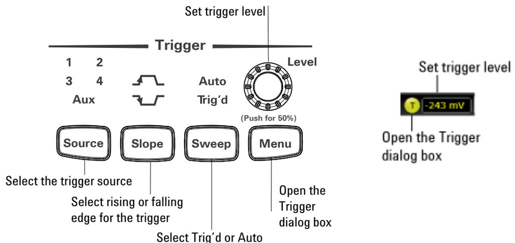
**Figure 20** Trigger controls and indicators
