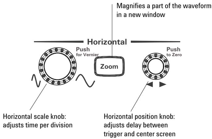
**Figure 16** Horizontal scale and position knobs, [Zoom] key
