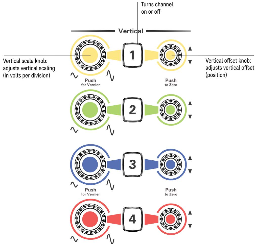
**Figure 18** Channel keys and vertical scale and offset knobs
