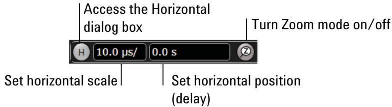
**Figure 17** User interface horizontal controls
