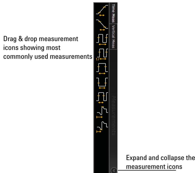
Figure 22 Drag & Drop measurement toolbar
