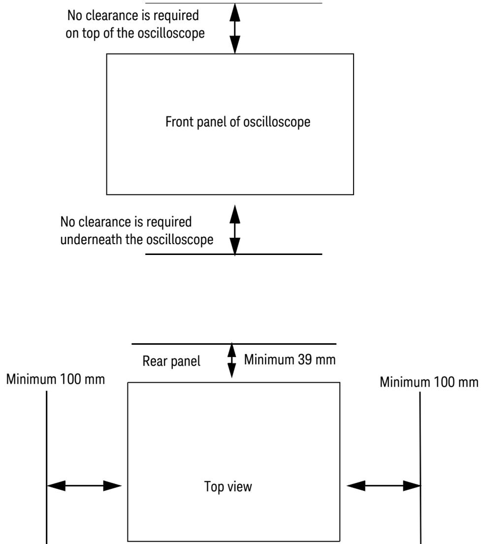
**Figure 1** Positioning the Z-Series oscilloscope with sufficient clearance
