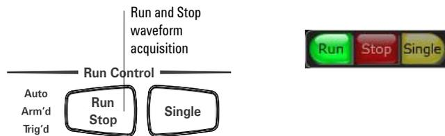
**Figure 15** Acquisition run control keys and buttons
