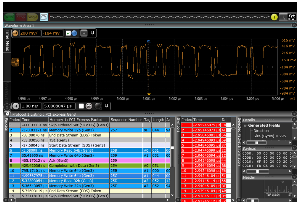
Z-Series decoding the PCI Express Gen3 packets.
