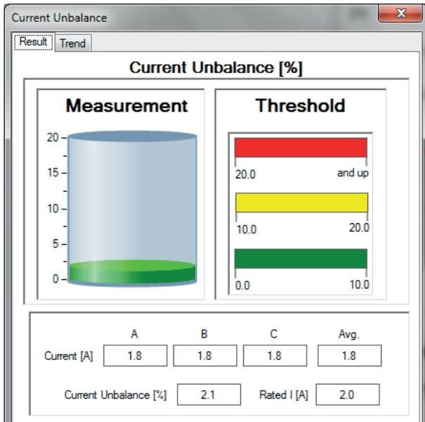
The EXP4000 provides views of various measurements with user-defined thresholds.
