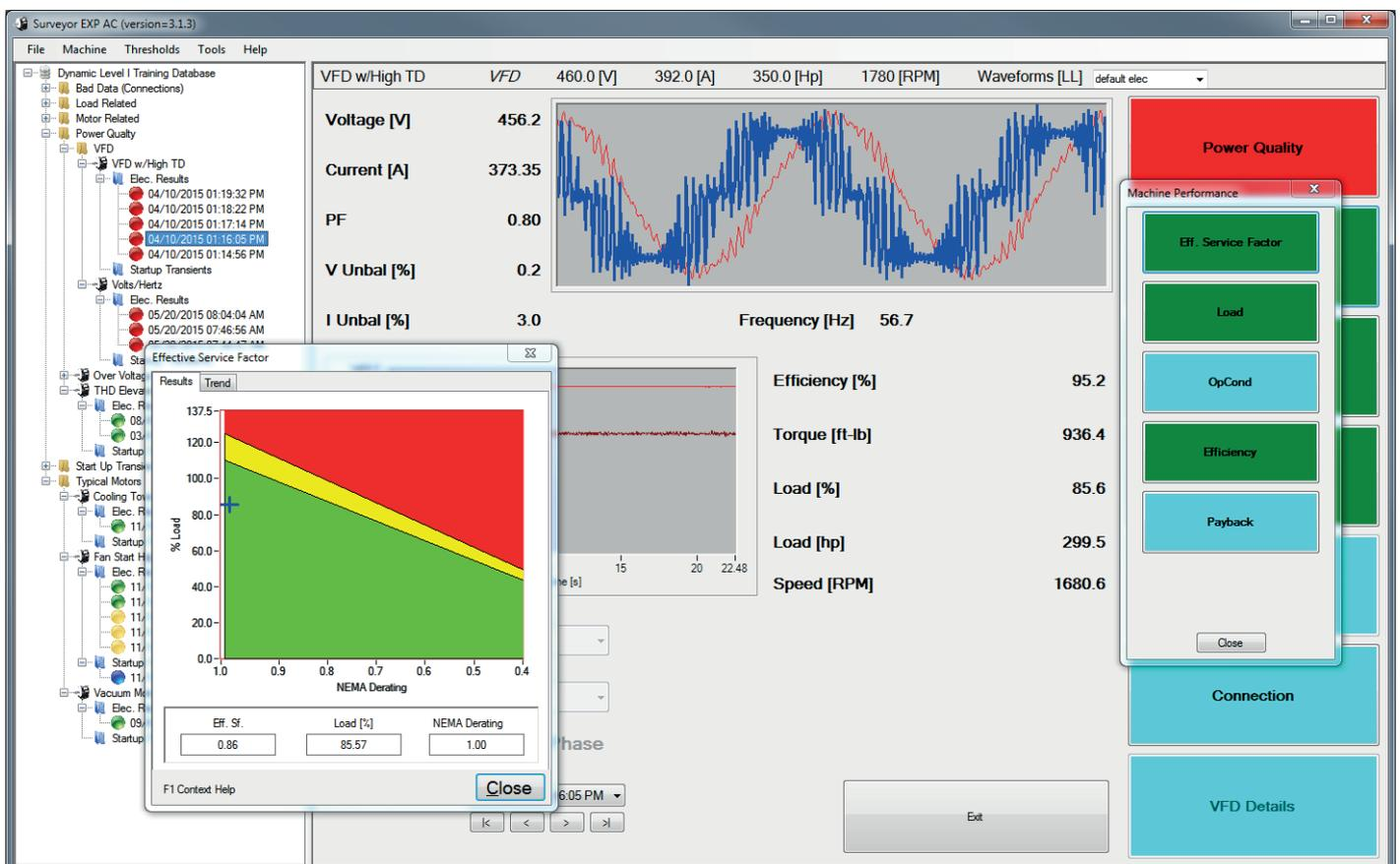
The user interface of the Baker EXP4000 dynamic motor analyzer features an at-a-glance summary of power, motor and machine condition.
