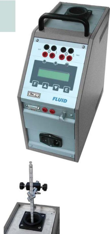
Fluid bath: aluminum, volume appr.  $400 \text{ cm}^3$ , homogeneity temperature via magnet-mixer, adjustable. Housing: metal; dimensions:  $160 \times 340 \times 330 \text{ mm}$ ; weight appr. 8 kg. Note: the stated accuracy is valid at ambient temperature  $+23^{\circ}\text{C}$  and is guaranteed for 1 year.
