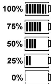
If the battery symbol drops to two bars the batteries will need replacing.
